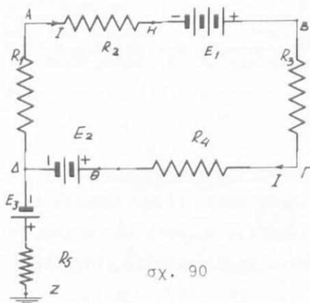
$$E_1 = 30 \text{ V}, E_2 = 20 \text{ V}, E_3 = 10 \text{ V}, R_1 = 20 \Omega, R_2 = 5 \Omega, R_3 = 6 \Omega, R_4 = 9 \Omega \text{ καί } R_5 = 10 \Omega.$$
