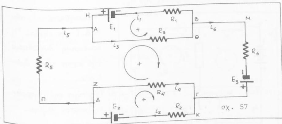
Δίδονται:  $E_1 = 8\text{V}$ ,  $E_2 = 16\text{V}$ ,  $E_3 = 12\text{V}$ ,  $R_1 = 2\Omega$ ,  $R_2 = 4\Omega$ ,  $R_3 = 4\Omega$ ,
