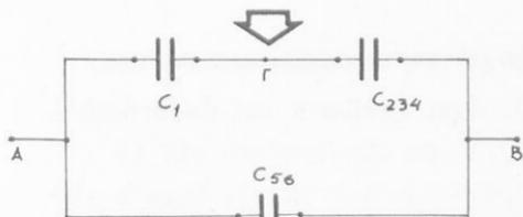
$$\begin{aligned} \text{ή } C_0 &= \frac{(\frac{C_2 \cdot C_3}{C_2 + C_3} + C_4)C_1}{C_1 + \frac{C_2 \cdot C_3}{C_2 + C_3} + C_4} + \\ &+ \frac{C_5 C_6}{C_5 + C_6} \quad \blacktriangleleft \quad (5) \end{aligned}$$
