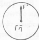
Σχ. 73. Ὁ λίθος ἐξασκεῖ ἐπὶ τῆς \Gamma\eta ς ἔλξιν F' , ἴσην καὶ ἀντίθετον πρὸς τὴν F .
