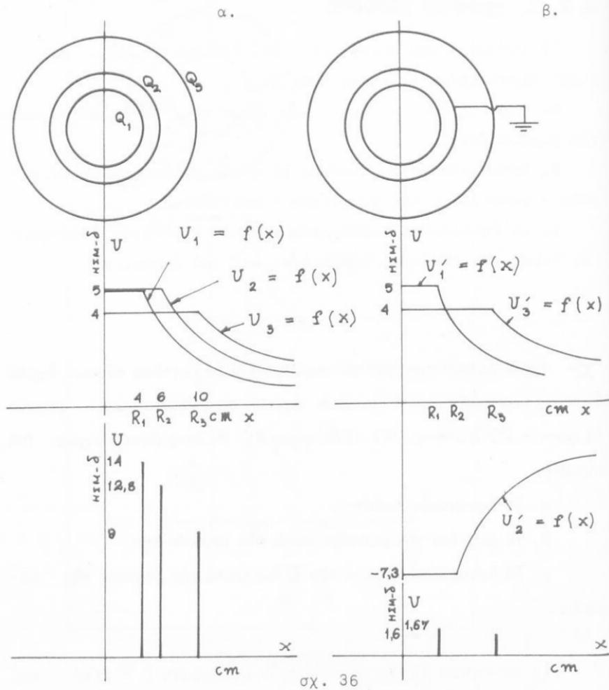
$$\beta. \quad U'_2 = \frac{Q_1}{R_2} + \frac{Q'_2}{R_2} + \frac{Q_3}{R_3} = 0 \quad (\text{λόγω γειώσεως})$$
