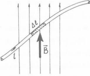
The diagram shows a curved conductor segment of length  $\Delta l$  within a magnetic field  $\vec{B}$ . The segment is oriented at an angle  $z$  relative to the direction of the magnetic field. Arrows indicate the direction of current flow along the conductor and the direction of the magnetic field.
