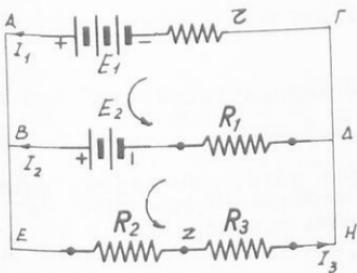
$$E_1 = 50V, E_2 = 20V, R_1 = 10\Omega, R_2 = 8\Omega, R_3 = 4\Omega \text{ καί } r = 2\Omega.$$
