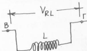
$$I_L = \frac{V_{RL}}{R_L} \quad (4)$$
