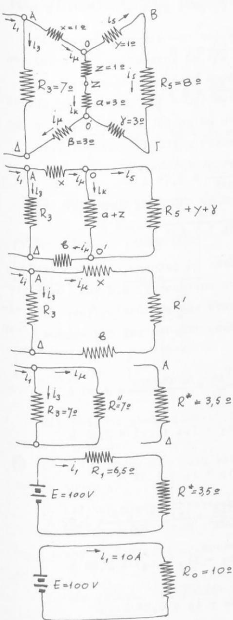
$$z = \frac{R_6 R_7}{R_2 + R_6 + R_7} = 1 \Omega$$
