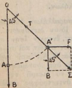
τὸ Πυθαγόρειον θεώρημα εἶναι  $(A'\Sigma)^2 = (A'B)^2 + (B\Sigma)^2$  ἢ  $\Sigma^2 = 4^2 + 4^2 = 4^2 \times 2$  καὶ  $\Sigma = \sqrt{4^2 \times 2} = 4 \times \sqrt{2} = 4 \times 1,414 = 5,656 \text{ kgf}^*$ .
